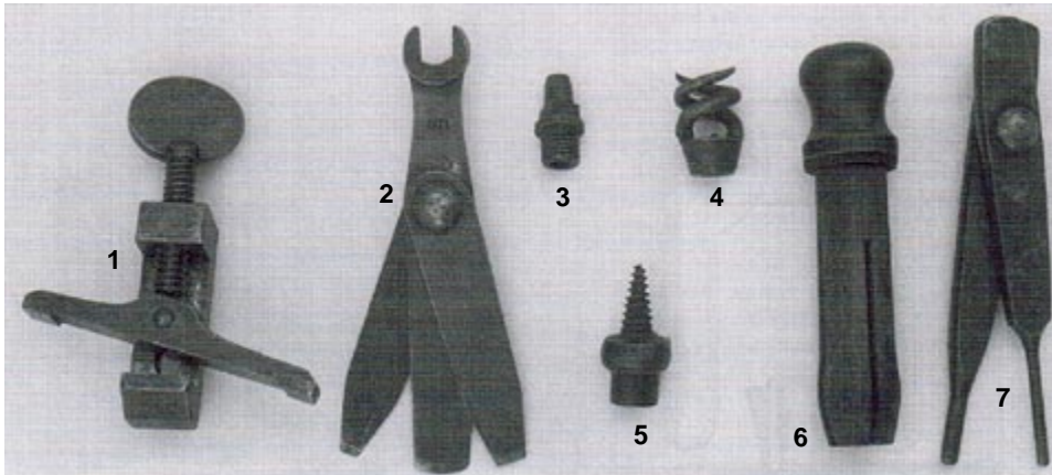
Musket tools as issued with the U.S. Army's .58 caliber Springfield rifles. 1 is the mainspring vise, 2 is the M1855 combination cone wrench and screwdriver, 3 is the spare cone, 4 is the wiper, 5 is the ball screw, 6 is the tompon, and 7 is the tumbler and spring punch, or drift.
