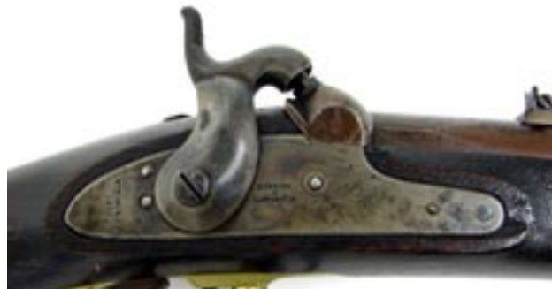
A view of the lockplate, with "HARPERS FERRY" stamped behind the hammer, and "U.S." and eagle stamped in front.
