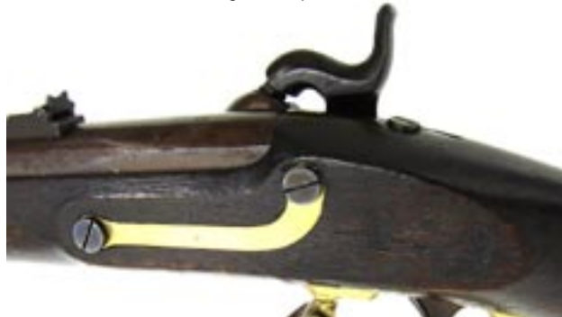
A look at the weapon's left side. Note the flip-up long range sights; this is the "late" version of the M1855 rifle sight.
