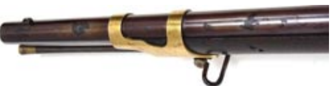
An overview of the barrel, showing the rear long-range and front blade sights, as well as the "long" upper barrel band.
