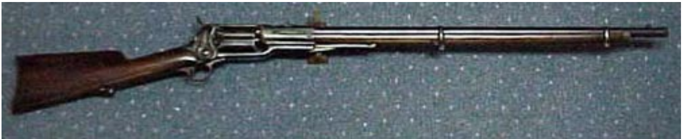
The Model 1855 Colt Revolving Rifle. The rifle was .56 caliber, and the cylinder held five shots. The Model 1856 could be fired as fast as the shooter could thumb back the hammer and aim at his next target. Reloading took some time, as each cylinder had to be recharged in the same manner as the Colt revolver handguns. For sheer firepower in a short time, the Colt Rifle was a formidable weapon in gaining fire superiority over an enemy armed with single-shot muskets or shotguns.
