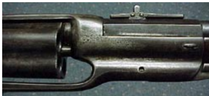
Closeup view of the front of the cylinder, showing the similarity of the rifle to the Colt revolver. Like the revolvers, the M1855 was sometimes subject to chain-firing, and the gap between the cylinder and the barrel often made it uncomfortable for the shooter who tried to rest the forearm in his left hand in the traditional firing stance.
