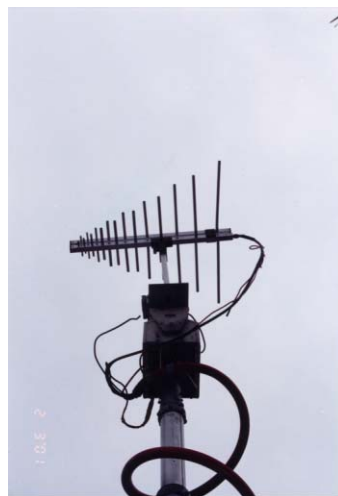
Figure 4 (left) the log-periodic antenna that was used and (right) its measured radiation pattern at 593 MHz, HP
