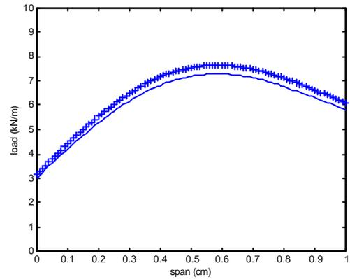
FIGURE 3. Static load estimated in the presence of 5% measurement noise (+) as compared to no noise case (-)
