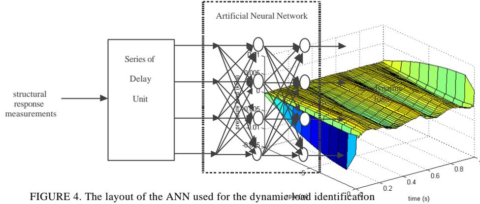
FIGURE 4. The layout of the ANN used for the dynamic load identification
