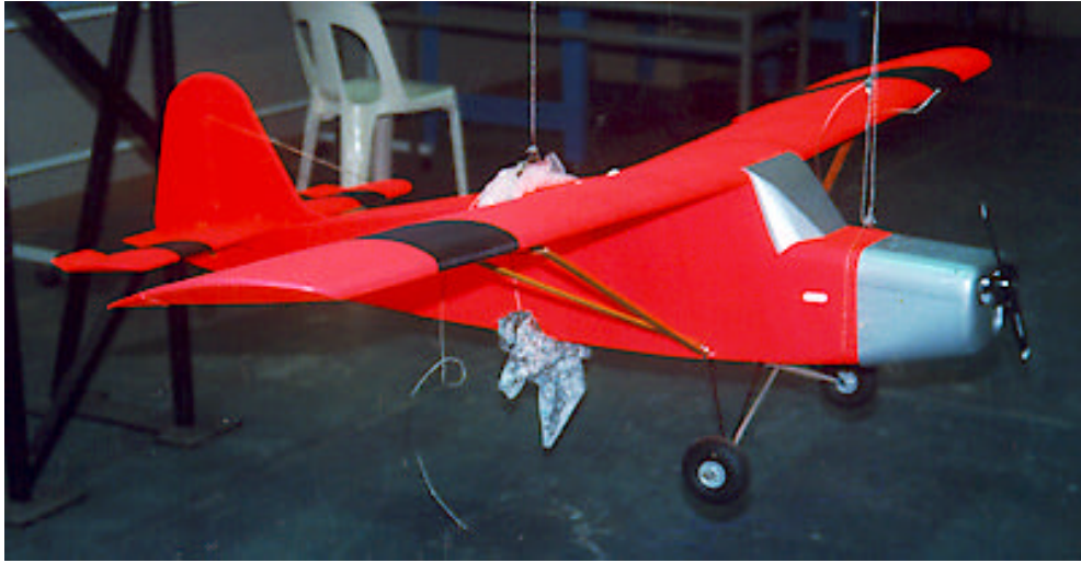
Figure 5-9: Experimental set-up to determine yaw and roll inertias
