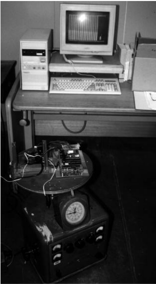
Figure 6-1: Rate gyro calibration using a rate table
