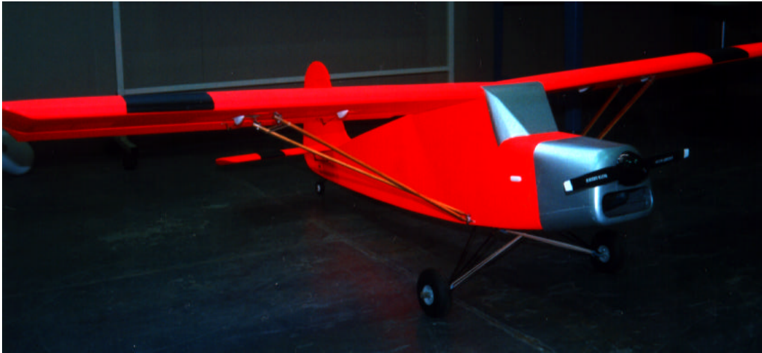
Figure 5-1: The Telemaster T240 aircraft model to be flight tested.
