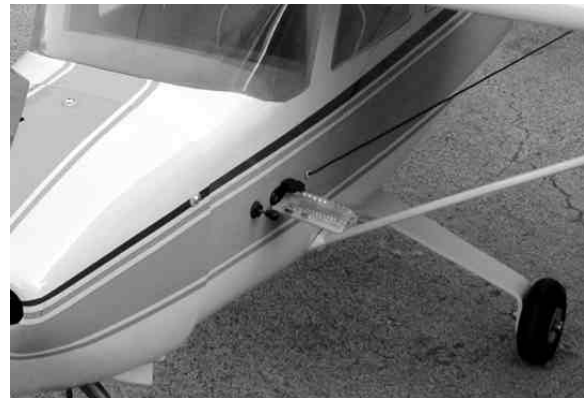
Fig. 10 Battery check on the author's Pica Cessna 182 using the external charge jack. Note the protective clear heat shrinking around the HOTCHEK (see text).
