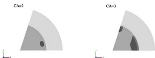
Figure 12: CFD predictions of soot formation, SOI=-5° aTDC
