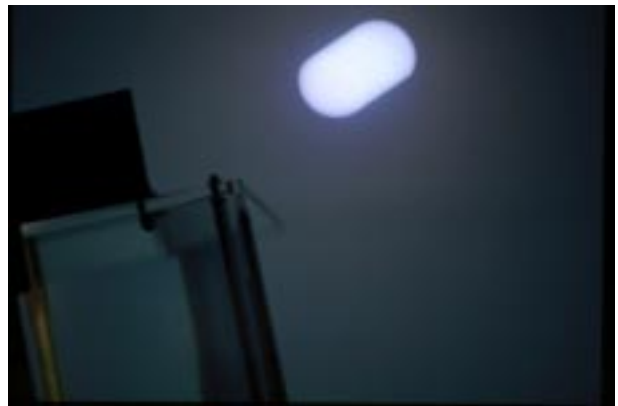
Figure 3: Testing the Fresnel lens under the 99% full moon. 1 May 1999, 21:20-21:35, Tokyo, Japan, at 35.5^\circ\text{N} . The lens is seen from its lower right side. The see through absorber, seen from its back, and almost filled out with light, appears in the lower left corner of the picture.
