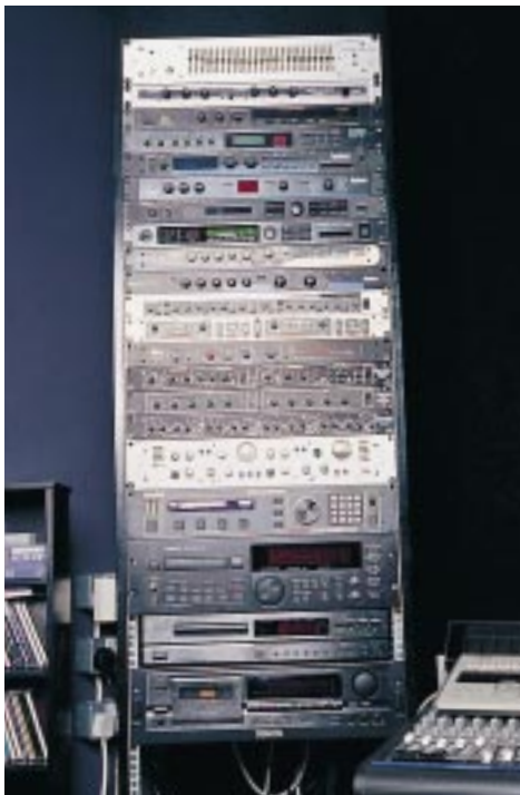
The extensive Dreamhouse processing rack, including the following: Urei graphic EQ, Aphex Aural Exciter Type C, Dbx 120x bass enhancer, Kawai RV4, Lexicon PCM80, Roland SDE330, Yamaha SPX990 and Zoom Studio 1201 multi-effects, Drawmer MX60 voice channel, Dbx 160A and Drawmer DL241 comp/limiters, Drawmer LX20 dual expander/compressor and DS404 Quad gate, TL Audio Ivory Dual Valve Compressor, Eventide H3000 UltraHarmonizer, plus Tascam DA30 MkII DAT, Denon CD player and tape deck.
